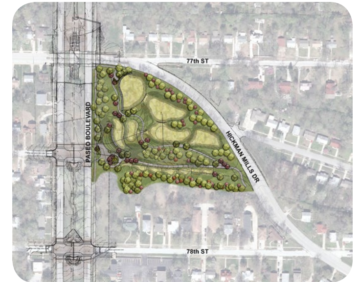
Final Plan: Digital plan showing vegetation and site layout with topographic information. (Rendering by Burns & McDonnell)
