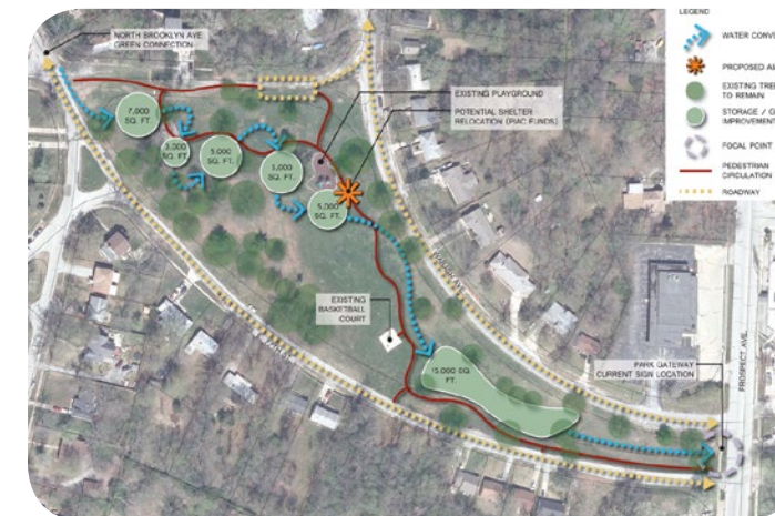
Final Site Diagram: Digital drawing showing site GSI layout and context. (Rendering by Burns & McDonnell)
