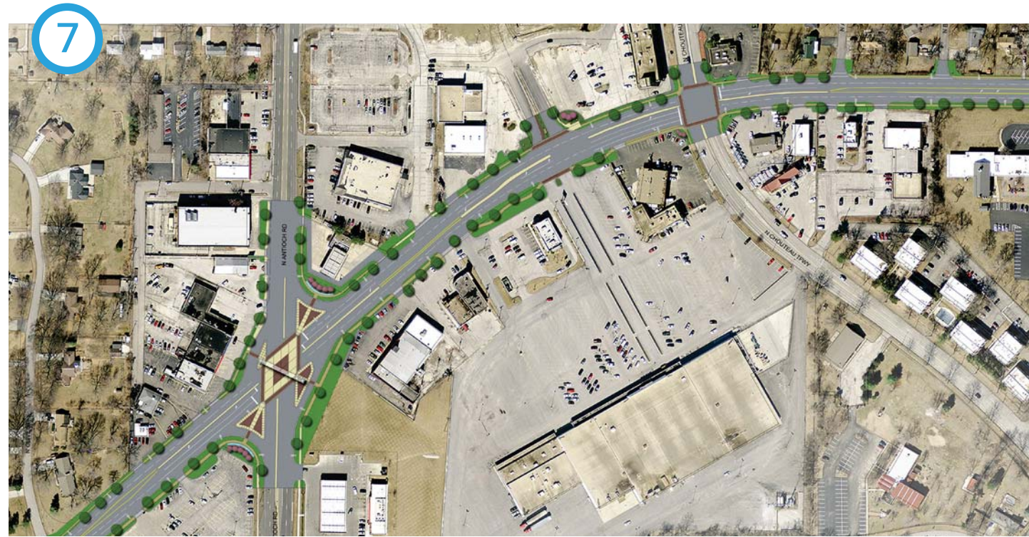
To improve traffic flow and reduce conflict points along the corridor, as many as five access points should be eliminated near the intersection of Antioch Road and Vivion Road. Similarly, two access points should be removed at the southeast corner of the Vivion Road and Chouteau Trafficway intersection.
