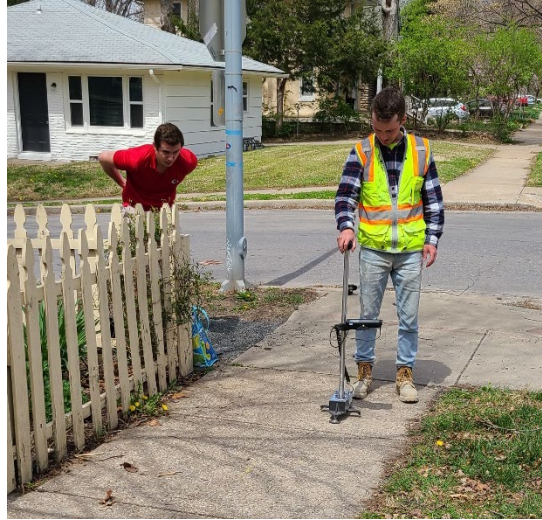
Figure 3. Dipstick profile testing for flatness
