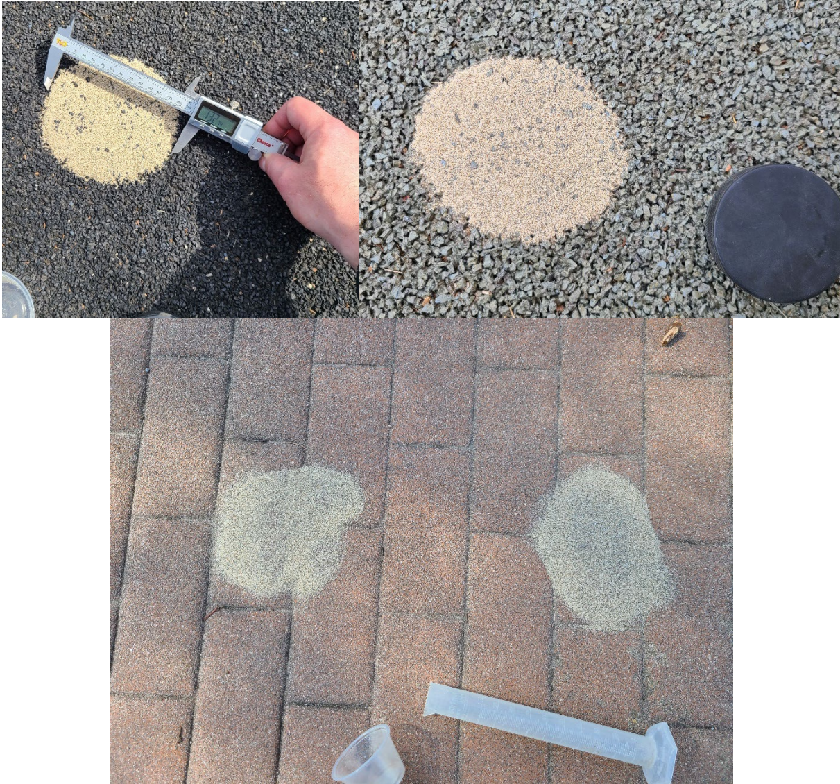
Figure 2. Sand patch testing for macrotexture (Top left rubber path, Top right Rubberway, Bottom left stamped brick tested over joint, Bottom right stamped brick tested between joints)
