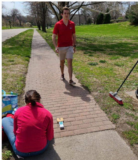
Figure 4. Biomechanical gait testing on the stamped brick test section
