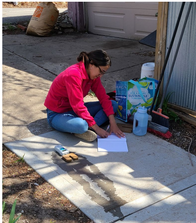
Figure 1. Drag meter testing for friction and microtexture
