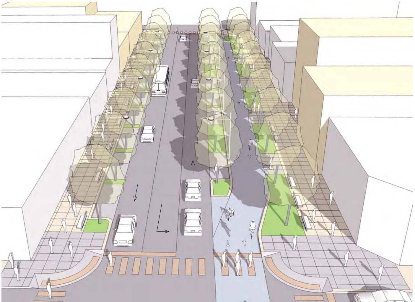
Perspective 2.2: Concept through the Crossroads District - Maintains two through lanes, a left turn lane, a protected bidirectional bicycle route and an enhanced pedestrian zone on the east side.
