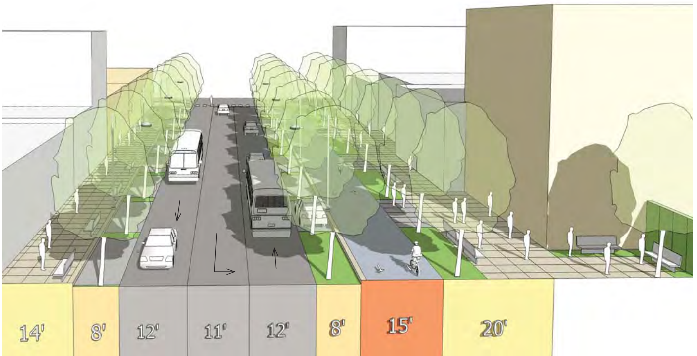
Section 2.2: Shows the typical dimension for areas within the Crossroads District with a 100' Right of Way.
