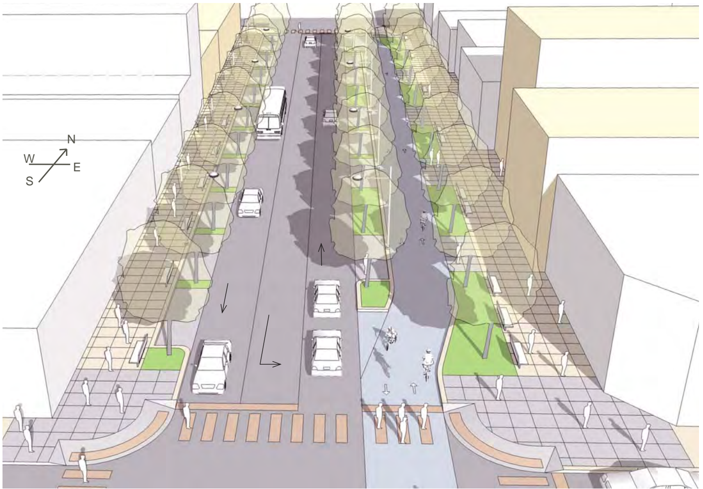
This is a perspective of the traditional redeveloped vision for Grand Boulevard. It includes an offset centerline creating additional pedestrian amenity zone on the east side of Grand. Within this zone is a bidirectional bike facility. Three lanes are proposed throughout the corridor. An additional fourth lane is commonly added for the block preceding the highway bridges.
