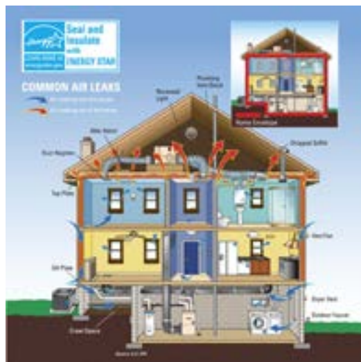
Common Air Leak Points in the Home Envelope 14
