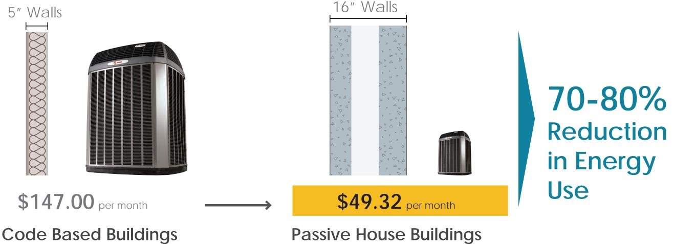
Poorly insulated building envelopes require oversized mechanical systems that consume 5x more energy than Passive House buildings.
