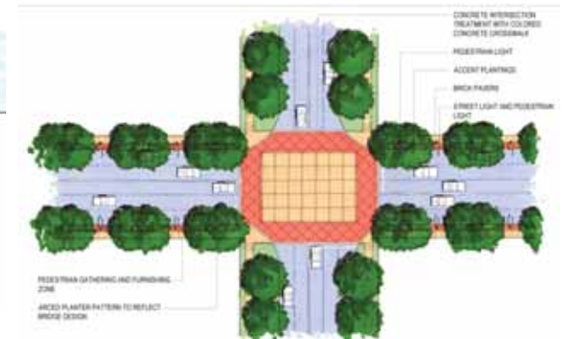
Major intersection pavement treatment
